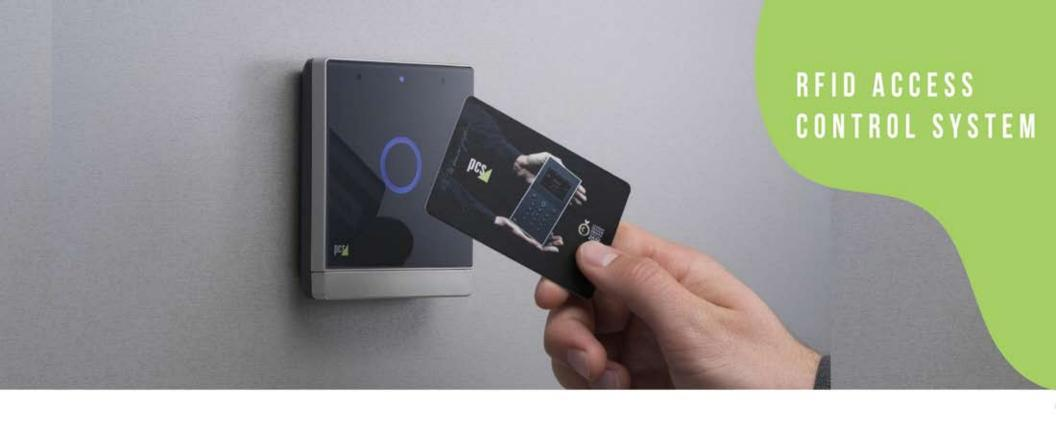
A radio frequency identification (RFID) device serves the same purpose as a barcode or a magnetic strip on the back of a credit card. It provides a unique identifier for the project. This method utilizes radio waves to transfer data between the RFID reader and the tags that's embedded in the product.
